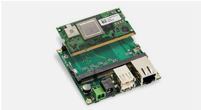
Abb. 1: Embedded Computer von Toradex (oben SoM, unten Carrier Board)
